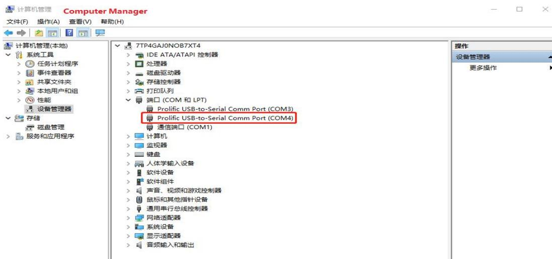
2. Open the computer serial port tool, set the serial port parameters: baud rate 115200, 8 data bits, 1 stop bit, no parity, no flow control, and open the serial port.
