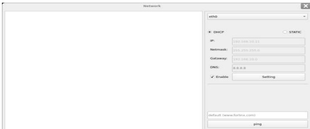
Check DHCP, select the NIC device needing to be configured, and click Apply and Restart Network at the bottom of the interface to restart the network and get the ip automatically.
